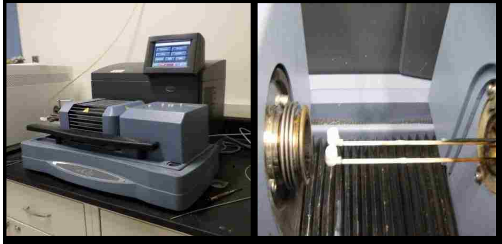
Figure 3.18: TGA/DSC SDT Q600 apparatus, and specimen holder.
