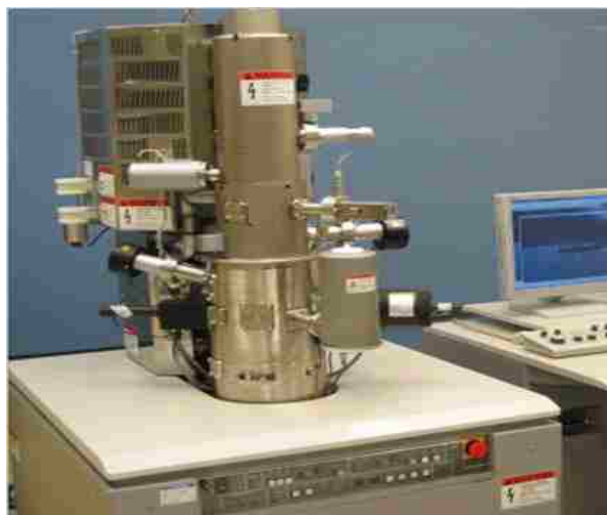
Figure 3.23: Hitachi S-5200 Scanning Electron Microscope apparatus.
