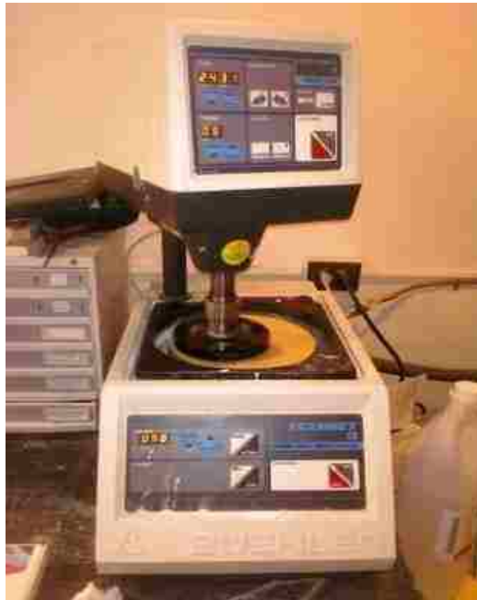
Figure 3.15: Polishing apparatus for preparation on nanoindentation samples
