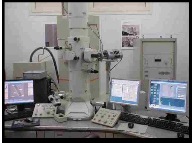
Figure 3.22: JEOL 2100F Transmission Electron Microscope apparatus.
