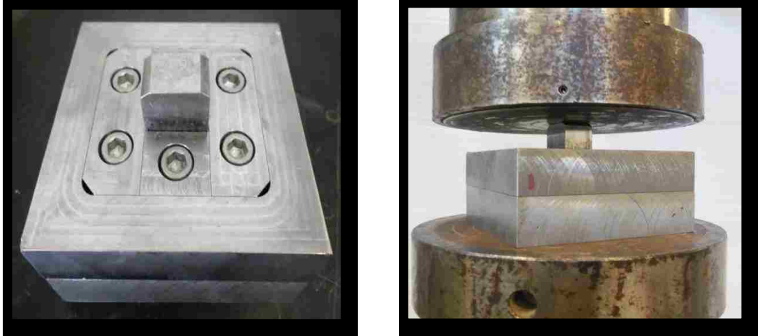
Figure 3.6: Compaction Apparatus and compaction loading
