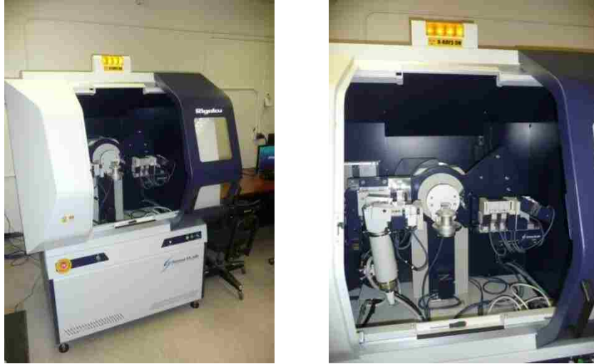
Figure 3.20: Rigaku SmartLab XRD testing system
